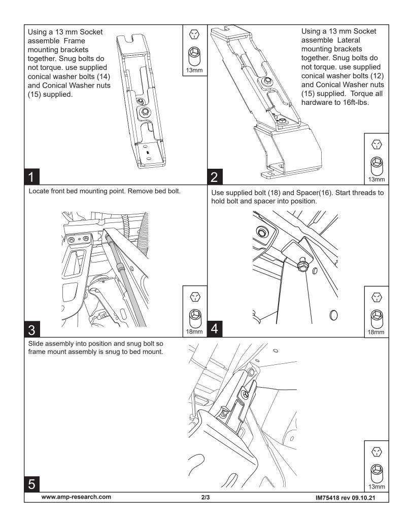
Install support brackets as shown below. Driver side (8) and passenger side(7) specific brackets are made. Discard extra bracket after install. Use supplied M8 conical washer bolts (14) and conical washer nuts. (15)
